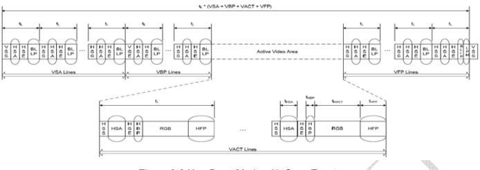
Figure 9-2 Non-Burst Mode with Sync Events
