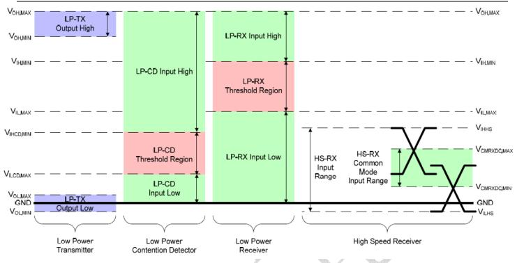
Figure 5-1 DSI signaling and Contention Voltage
